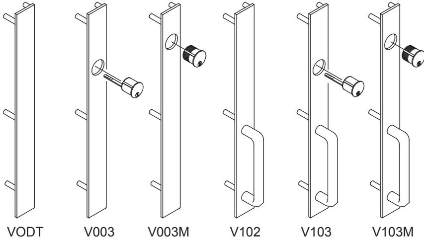
Note: For use of cylinders over 1 3/8" in length, a spacer ring is required on exterior side of trim.
