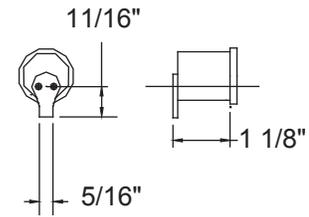
Note: If door is less than 2 1/4" thick tailpiece will have to be cut down.
