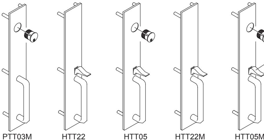
On 22M and 05M trims, thumb piece is held in place by a band for shipping. Remove prior to installing trim in door. Thumb piece will remain in place once installed.
